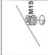
Step 4: Using screwdriver or Allen wrench twist cam clockwise.
